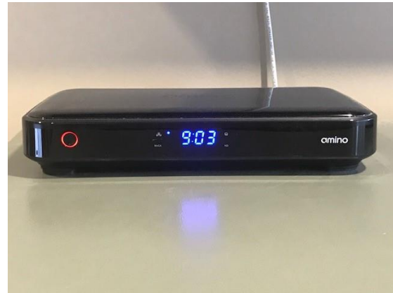
DVR Cable Box (Power Off - Red Light)
